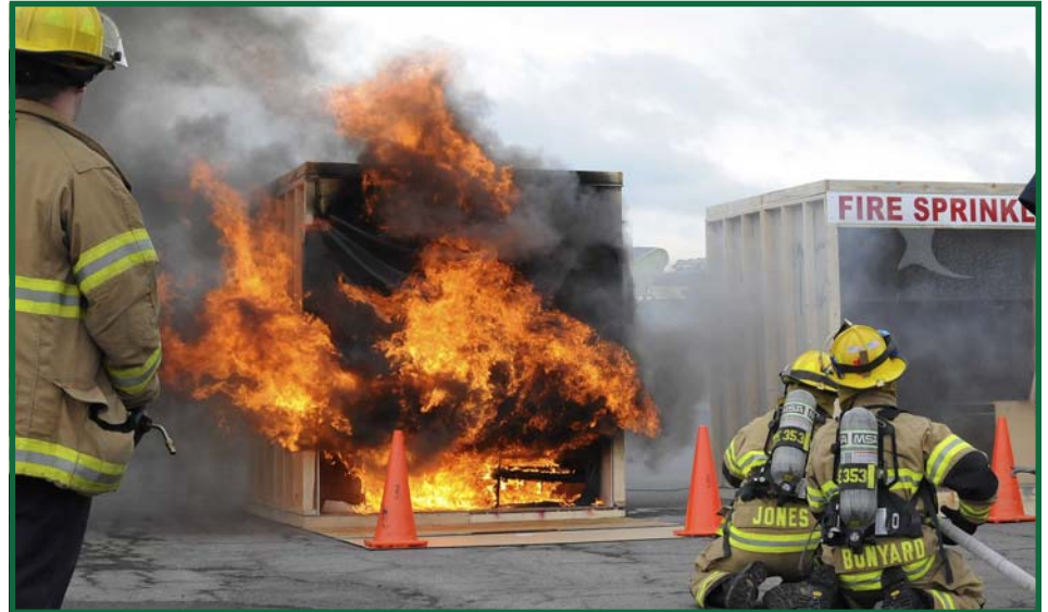
BST&G fire personnel demonstrate the differences in a fire sprinkler and a non-fire sprinkler environment. The fires were set at the same time in both rooms.
