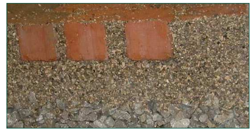
This cross section shows how Walnut St. will be designed to better handle storm water to protect local water resources.
